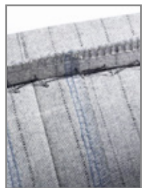
6. Hemming double blind stitch on skirts, unlined or half-lined jackets Class 352
